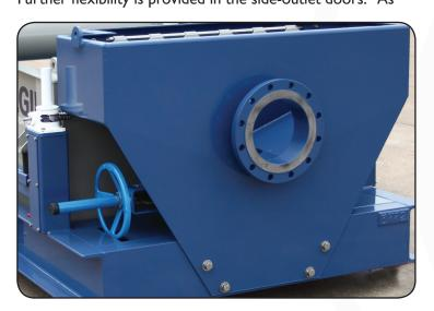
a standard feature, the side discharge doors incorporate mounting faces. The mounting configuration also allows for a host of standard discharge adapters to be mated to the shaker side outlets.
